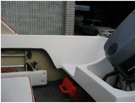
Foam can be fitted under the outboard well and deck mould
