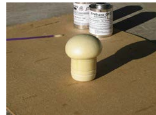
A small amount of liquid expands significantly
