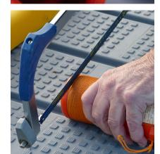
With a hacksaw, carefully cut around the base of the cylinder below the orange lanyard. Do not cut beyond plastic encasement.
