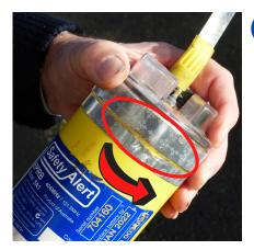
Break seal on reflective tape at top of EPIRB and unscrew anticlockwise. Do not accidentally turn EPIRB on.
