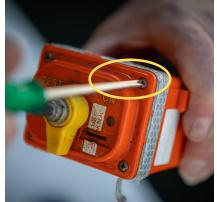
With a Phillips head screw driver, remove four screws at
