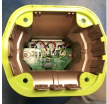
Remove the 2 screws circled in red and then remove the PCB from the EPIRB case. The 3 Lithium battery packs can then be removed from the EPIRB.
