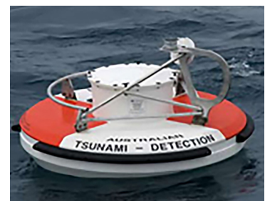
The surface component of an operational deep-ocean tsunami detection buoy
