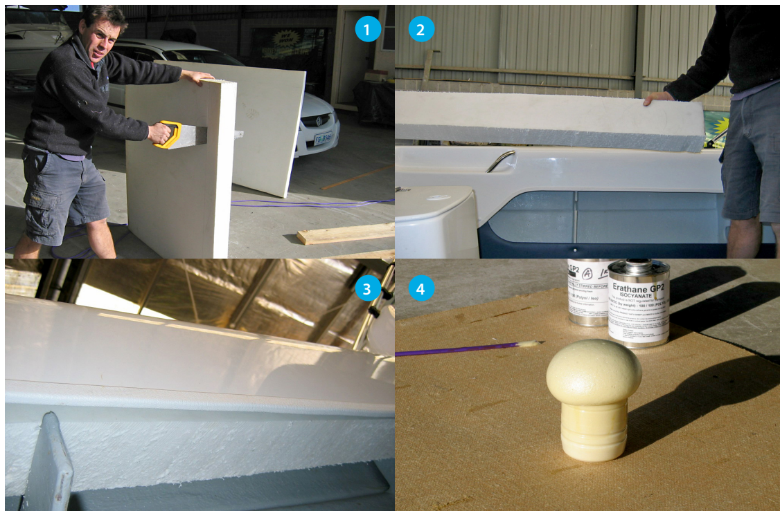
1. Most closed-cell foam is easily cut and shaped; 2. Microlen™ foam about to be fixed under gunwale; 3. Microlen™ foam now fixed in place; 4. Example of pouring foam expanding after mixing
