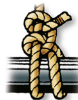
Round turn and two half hitches
